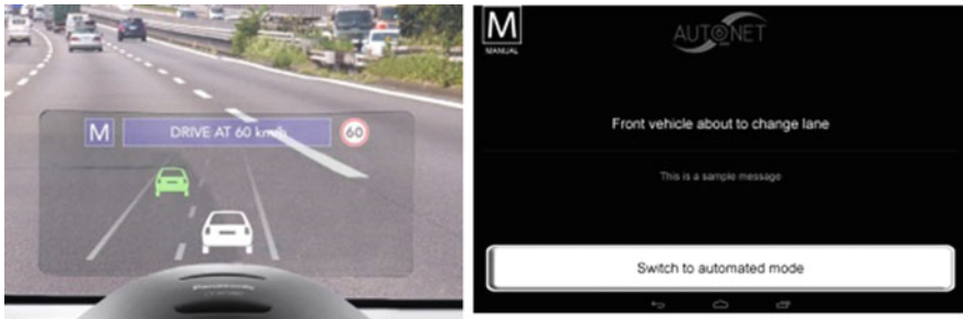
Fig. 26.1 Indicative screenshots of the dual-screen AutoNet2030 HMI system: HUD ( left ) and Android ( right )
